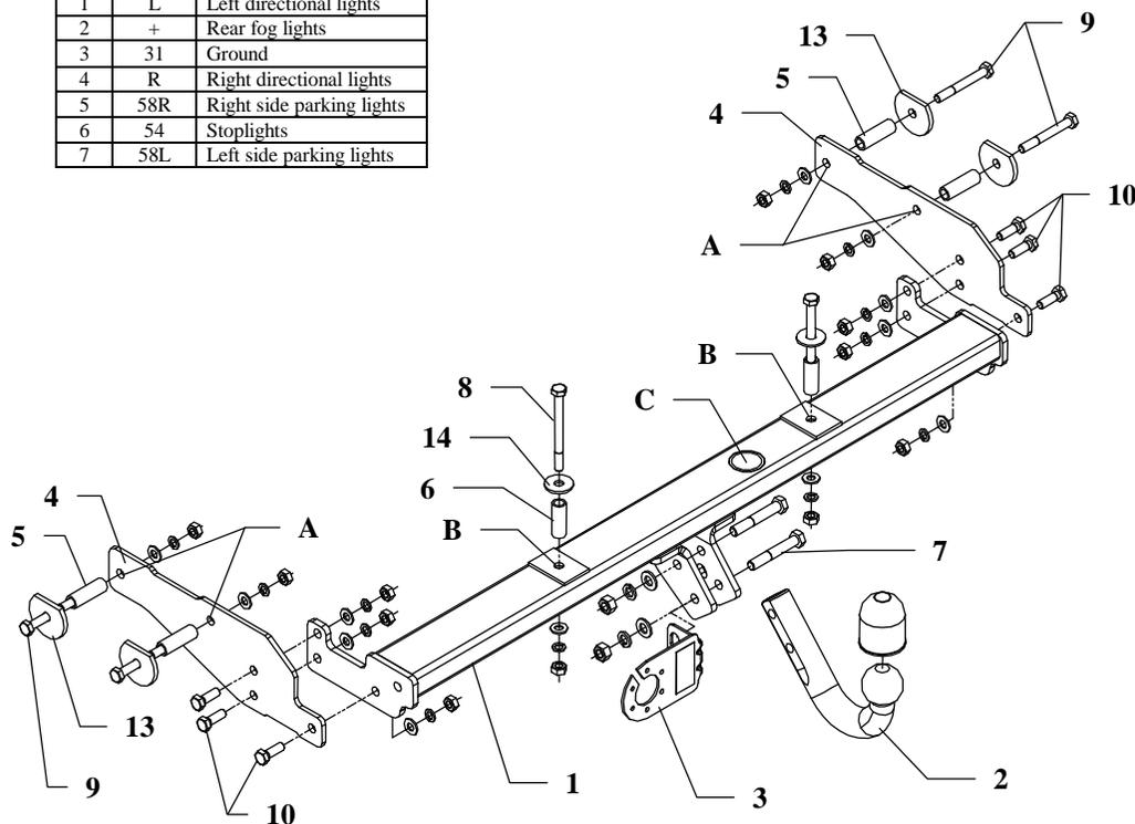
This towing hitch is designed to assembly in following car: **CITROEN C15**, produced since 1985 till 2007, catalogue no. **P06** and is prepared to tow trailers max total weight **900 kg** and max vertical load **45 kg**.
